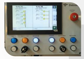
The RCS system is commanded by PLC automatic machine which controls multiple independent retractable catenary sections. The main control panel (master) is equipped with a LCD display with further control and signalling elements (slave). Retractable catenary can be controlled with the use of buttons on the LCD display. The display can be also used for system setting, its diagnostics and potential failure solving. The system enables remote monitoring and diagnostics.
