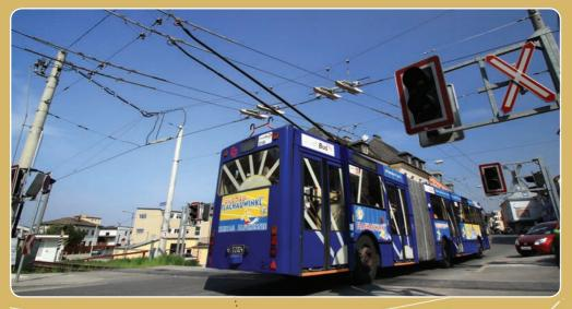
New type of TBUSxTRAM (15°-65°) crossings without interruption of electrical supply is perfectly silent and ensure vehicle's sustained passage with current.
