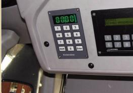
Using this code the vehicle pass automatically through all switches until its final destination.
